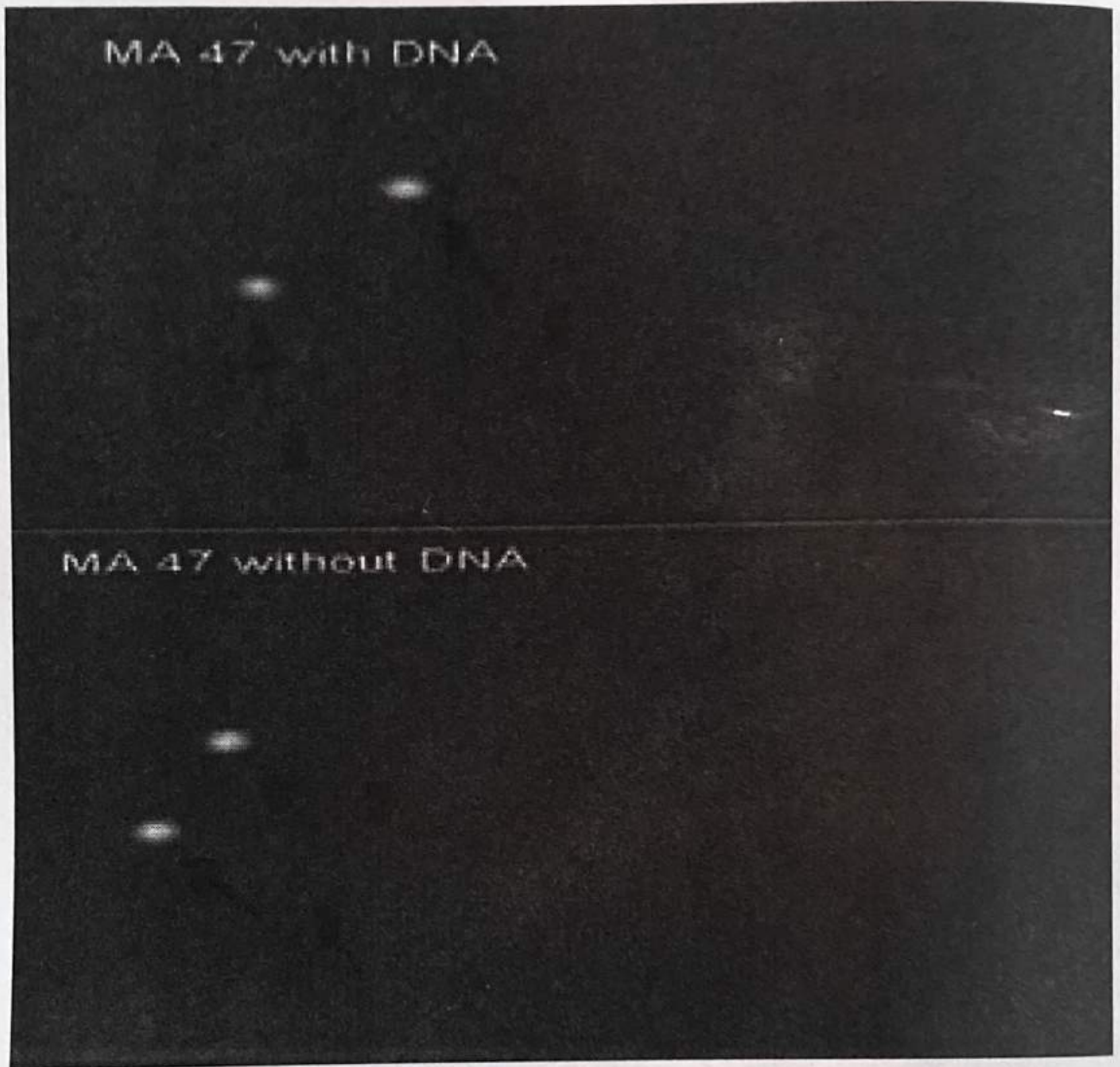
Figure 4. DNA-binding affinity of MA 47 extract in Two-dimensional Thin Layer Chromatography. [Arrows indicate locations of molecules in the second dimension both in the measuring (with DNA) and reference (without DNA) plates].
