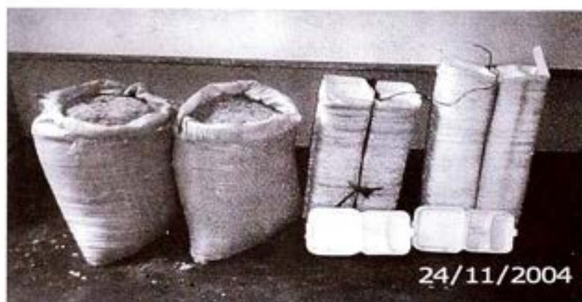
Figure 3.1. Dry Rice hull and Washed Polystyrene Foams
