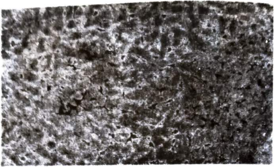
Figure 12. Kulintang sample with cored structure. Etchant: Ferric chloride
