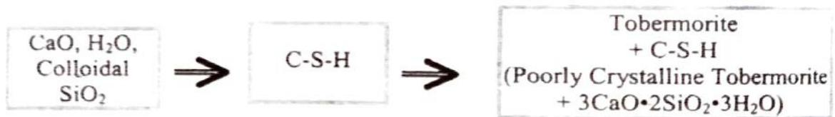
Figure 5. The Synthesis Reaction
