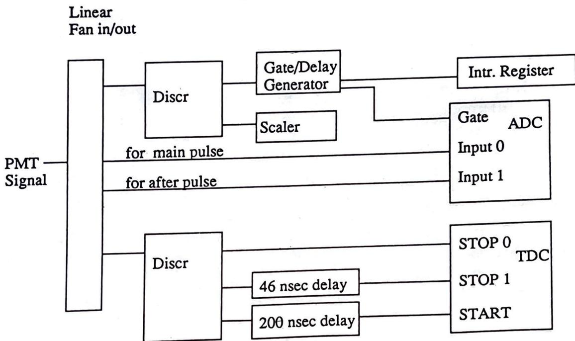
Figure 1. Electronics for the data acquisition used in the experiment.
