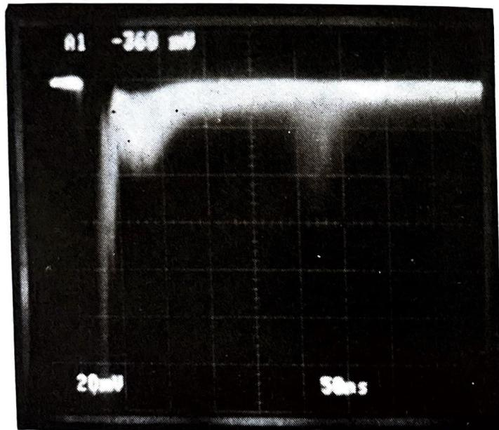
Figure 10. After 356 hours of 100% helium exposure. The afterpulse is remarkably present at a time of 250 ns after the main pulse.
