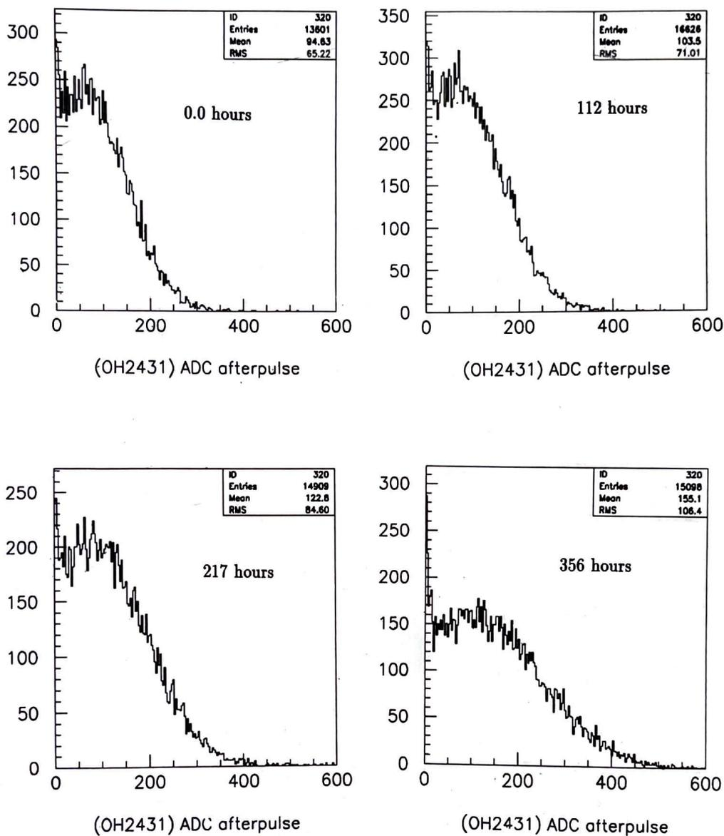
**Figure 13.** The ADC distribution for the conventional tube type (old) at different periods of pure helium exposure.
