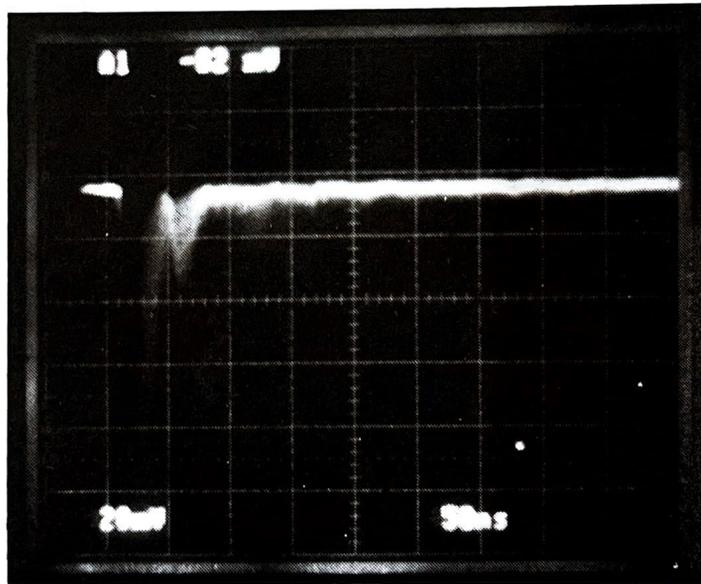
Figure 6. After 470 hours of pure helium exposure. Notice the afterpulse occurring 100 ns after the main pulse. (The scales are the same as the above figure.)
