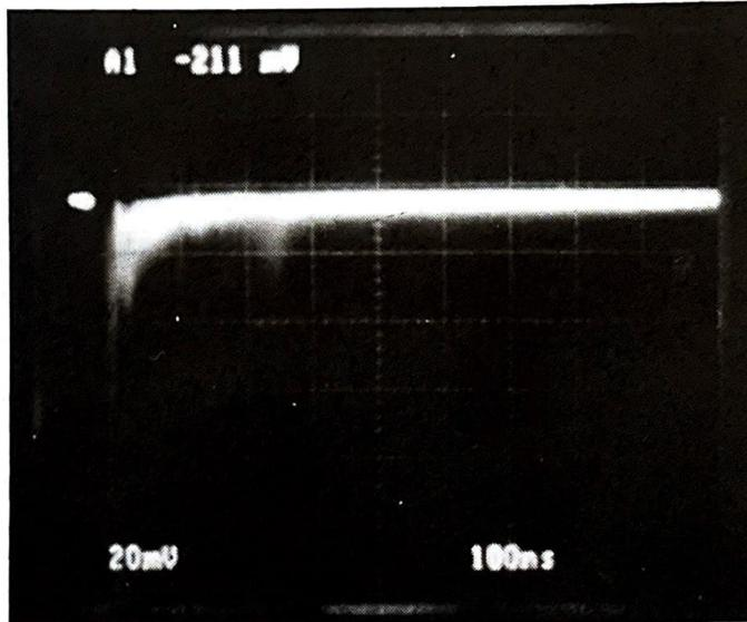
Figure 8. After 470 hours of helium exposure. The afterpulse can be seen about 250 ns after the main detector signal.
