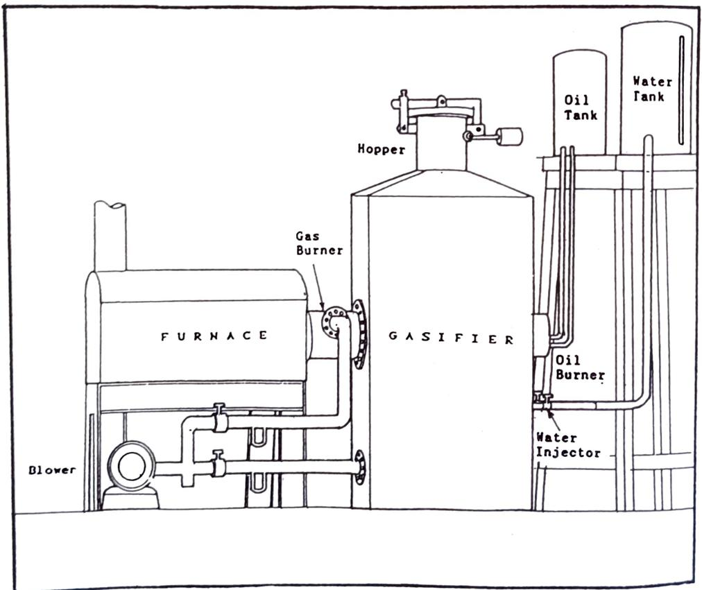
Figure 1 – Schematic Diagram of the Experimental DWIG Gasifier-Furnace Set-up
